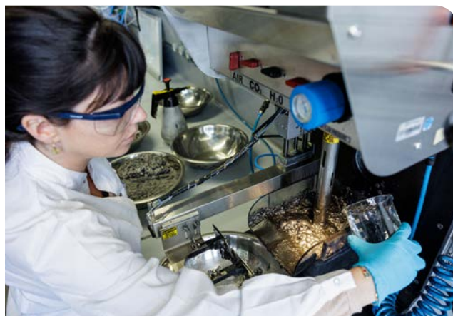
Dr. Anna Vanderbruggen at the froth flotation separator for recycling graphite
